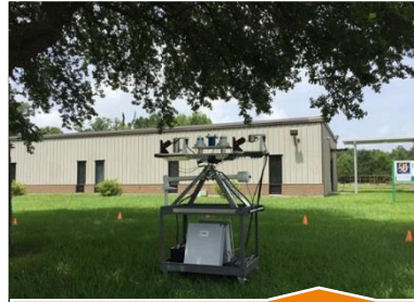
SU Ag Center's UV-B monitoring station built with help from the USDA-UVBMRP
