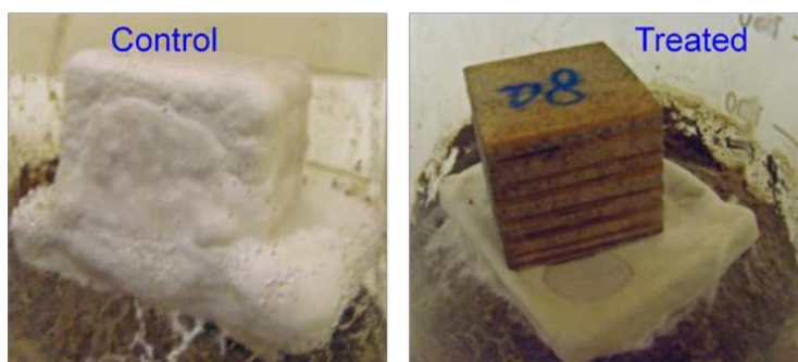
Figure 6. Wood treated with CCCSNs shows remarkable decay resistance against white rot fungus, Trametes versicolor , after 16 weeks of testing based on AWPA E10 Method (for Decay test).
