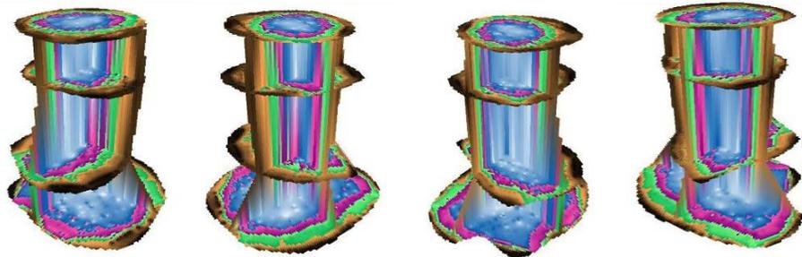
Figure 4. Illustration of water oak trunk decay pattern using Tree ID #1 (pictured in the bottom left), showing the two dimension (2-D) cross-sectional tomography images measured at four levels (15, 80, 130, 165 cm above ground) and 3-D images constructed after combining all 2-D images in four different directions.
