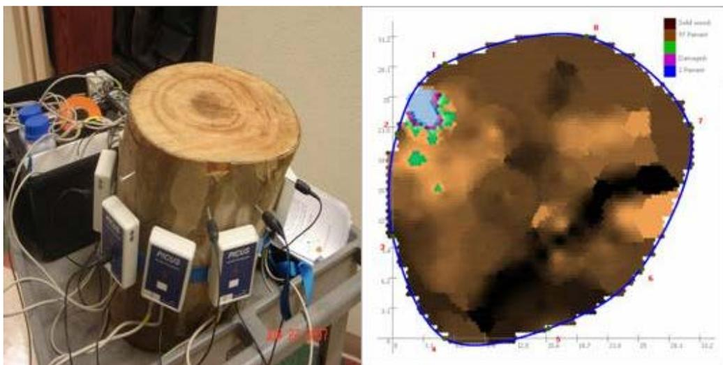
Figure 2. Another example of a test stump, showing 97% of the wood is solid (brown and black colors, 2% wood is damaged (blue/purple), and 1% of the wood is weakened (in green color). The circumference of the stump is 84 cm.
