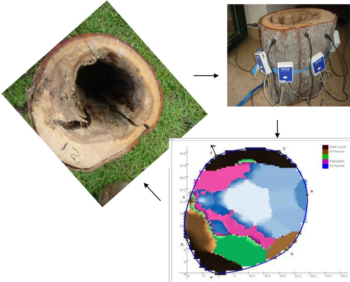
Figure 1. An example of a test stump showing how the Picus Sonic Tomography technology works. The image shows 61% decay wood (white, blue, and purple colors), 27% solid wood (black and brown colors), and 12% transitional wood (green color).
